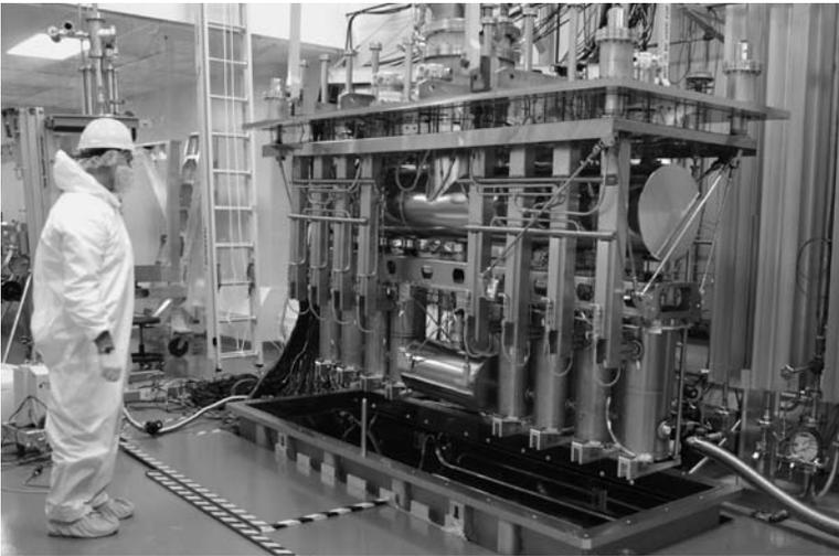
Cryomodule for the TRIUMF ISAC-II accelerator
