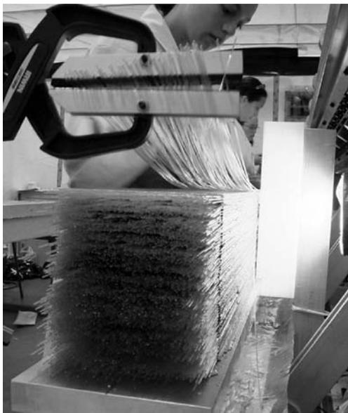
Scintillating fibres for the barrel calorimeter on the GlueX detector
