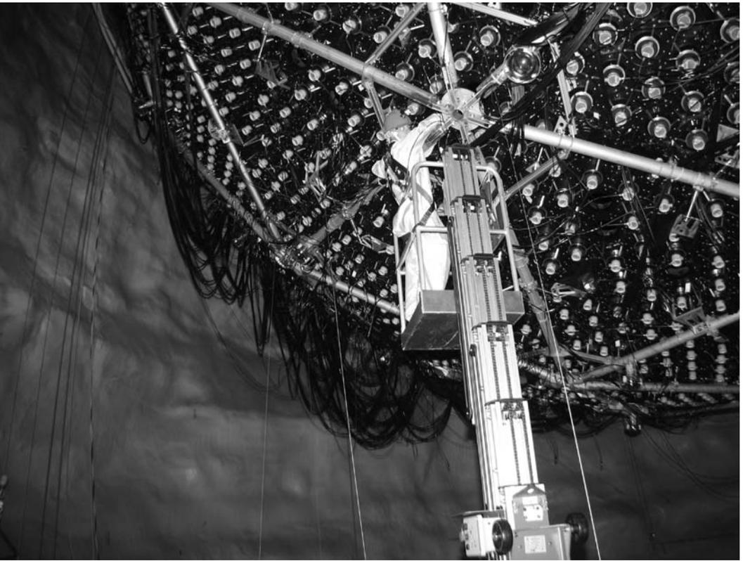
Upgrading the SNO detector for the SNO+ experiment
